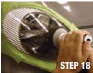
16. Continue using the same backer. Attach the white foam polishing pad to the 3" polishing tool.
