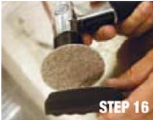
13. Apply a dime-sized amount of the heavy polishing compound to the yellow foam pad. Too much compound will result in excessive sling and added clean up. DO NOT run the foam pad dry.
