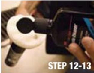
12. Remove the soft interface pad and attach the velcro backer plate for steps 12 - 18. Attach the yellow foam compounding pad to the 3" polishing tool.
