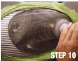
6. Continue using the same tool. Remove the P800 grit disc and attach the P1500 grit disc to the soft interface pad.
